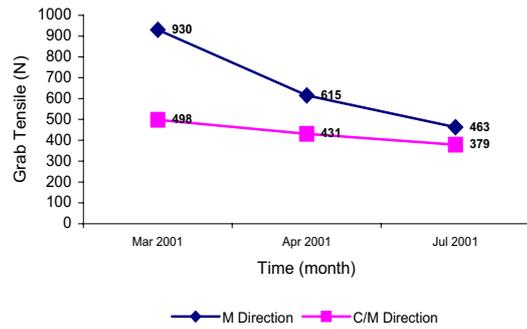
Figure 4. Grab Tensile Strength vs Time for Sample Sprayed with Roundup Herbicide
